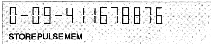
Figure D12. Display status during programming repertory number 0-AP-0-9-AP-4-1-1-6-7-8-8-7-6
