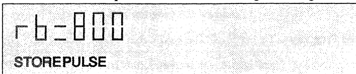
Figure D29. Display status at set impedance Rb, showing the Rb value of 800 ohm.
